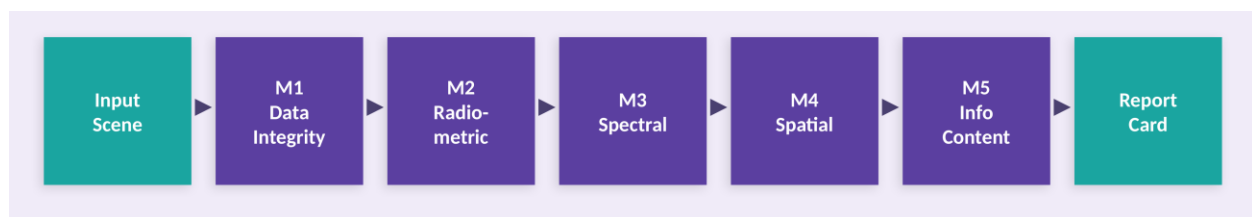
Figure 2. The C-CERT pipeline: an input scene runs through five independent modules (M1–M5) to produce a standardized report card. Modules can run alone or as a full pipeline [1].
